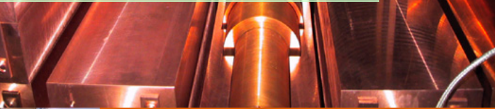
detectors during installation; in the central and right up detectors the new shaped Cu shield surrounding light guides (acting also as optical windows) and PMTs was not yet applied
